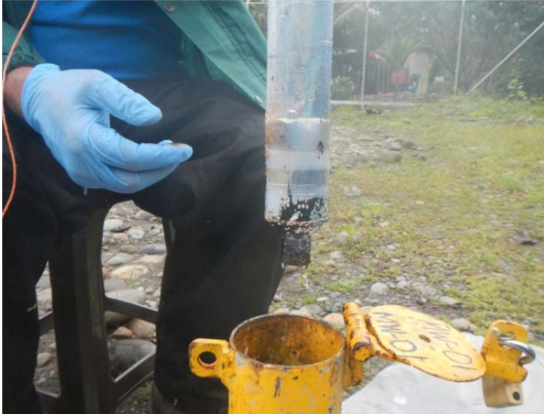
Figure RS-4: Photo of oil on LBG groundwater sample bailer from well MW-01
