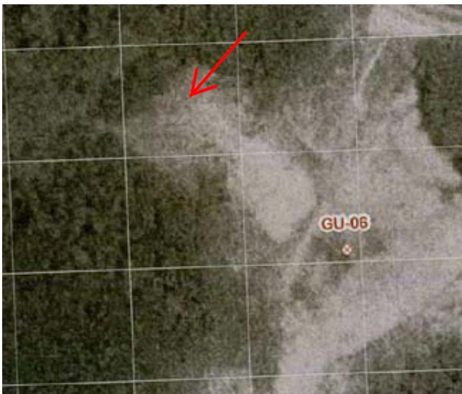
Figure RS-11: 1990 Aerial Photograph showing that the location of Pit A was cleared and graded; however, there is no indication of the flare structure. The presence of the cleared area on the 1990 photo, which becomes a densely vegetated area on the subsequent photos in 2001 (Figure RS-12) and 2004 (Figure RS-13), confirms the conclusion that Pit A was closed in 1990 and that the flare was subsequently constructed atop the closed pit.
