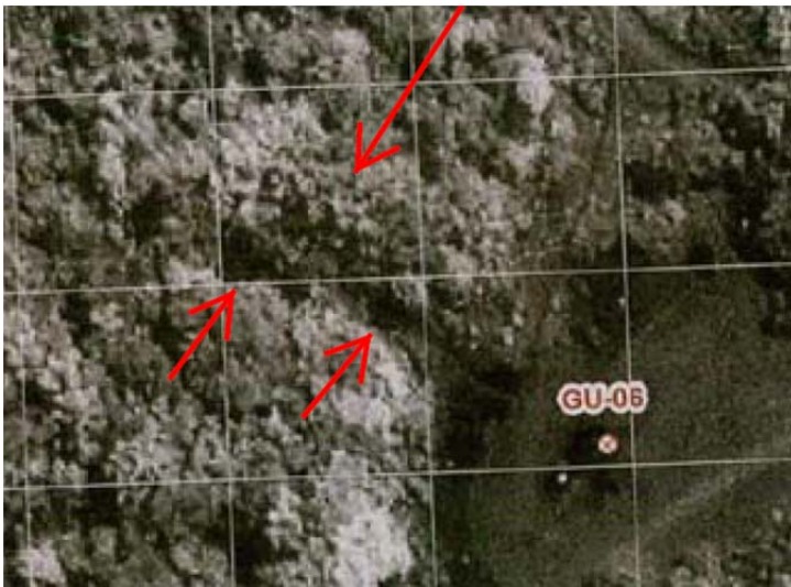
Figure RS-13: 2004 IKONOS Satellite Photograph (1 meter resolution, panchromatic image) showing the location of former Pit A (denoted by larger arrow) completely overgrown with vegetation. The two smaller arrows denote "tree shadows" and do not indicate surface impacts associated with former pits. The image coloration denotes vegetation.
