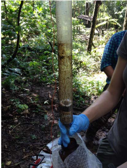
Figure RS-17: Oil on groundwater sample bailer from GU-06 Monitoring Well MW-4.
