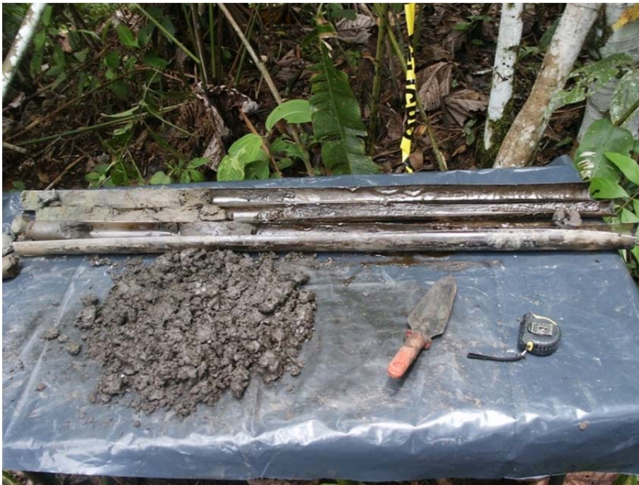
Figure RS-1: Photograph taken by Chevron of oil saturated sand in Pit 3 during their unofficial Pre-Inspection 16
