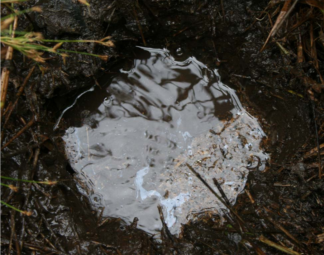
Figure RS-7: Borehole in sediment with oil droplets coming to water surface at SSF-25
