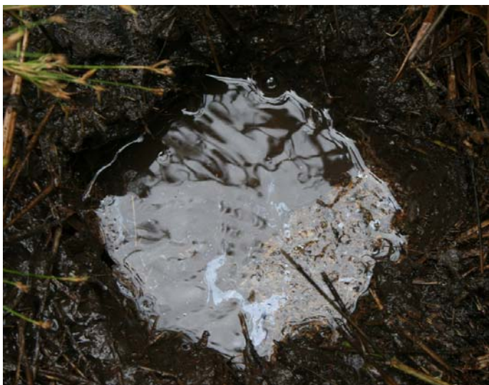
Figure 2.2-5 - Borehole in sediment with oil droplets coming to water surface at SSF-25
