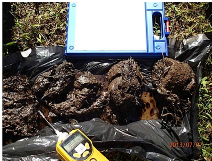
Figure 2.2-6 - Oil saturated sediment from wetland just north of YU-02
