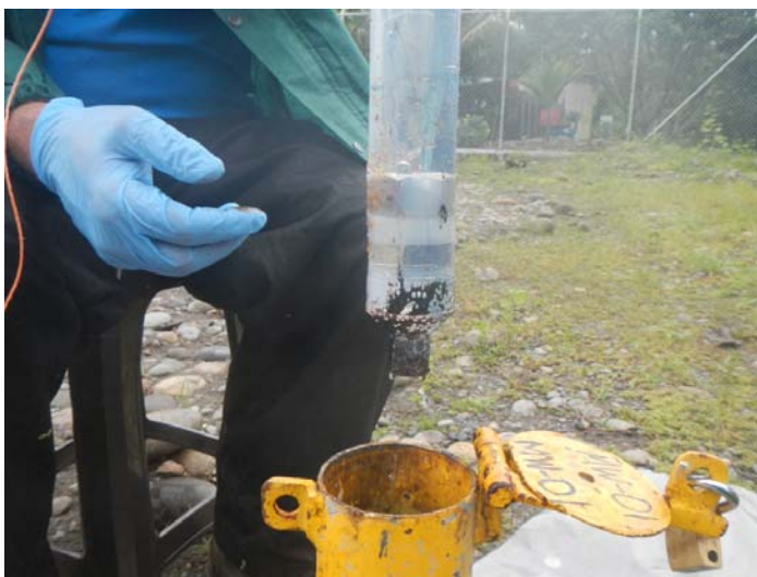
Figure 2.2-3 - Photo of oil on groundwater sample Bailer from well MW-01 taken during our site investigations
