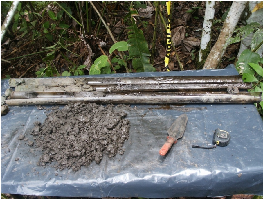
Figure 2.2-2 Photograph taken by Chevron of oil saturated sand in "Pit 3" during their unofficial Pre-Inspection 91
